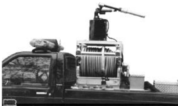
Figure 1 - High mount location of turret on top of Indiana slip-on unit.
